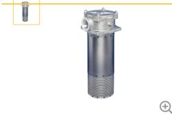
The TTF Series features pre-filtration by means of a magnet column and a quick response bypass with low hysteresis. Maximum pressure 10 bar. Maximum flow 500 l/min. A second return port is an available option as is a filling port in the filter cover.
