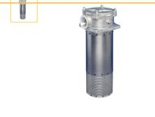
The TTF Series features pre-filtration by means of a magnet column and a quick response bypass with low hysteresis. Maximum pressure 10 bar. Maximum flow 500 l/min. A second return port is an available option as is a filling port in the filter cover.
