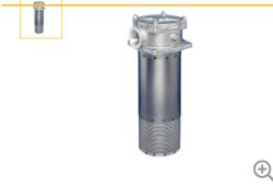
The TTF Series features pre-filtration by means of a magnet column and a quick response bypass with low hysteresis. Maximum pressure 10 bar. Maximum flow 500 l/min. A second return port is an available option as is a filling port in the filter cover.
