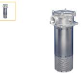
The TTF Series features pre-filtration by means of a magnet column and a quick response bypass with low hysteresis. Maximum pressure 10 bar. Maximum flow 500 l/min. A second return port is an available option as is a filling port in the filter cover.
