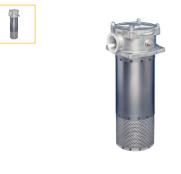
The TTF Series features pre-filtration by means of a magnet column and a quick response bypass with low hysteresis. Maximum pressure 10 bar. Maximum flow 500 l/min. A second return port is an available option as is a filling port in the filter cover.
