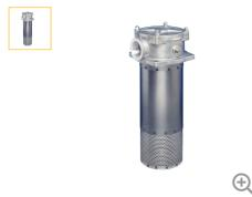
The TTF Series features pre-filtration by means of a magnet column and a quick response bypass with low hysteresis. Maximum pressure 10 bar. Maximum flow 500 l/min. A second return port is an available option as is a filling port in the filter cover.
