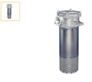
The TTF Series features pre-filtration by means of a magnet column and a quick response bypass with low hysteresis. Maximum pressure 10 bar. Maximum flow 500 l/min. A second return port is an available option as is a filling port in the filter cover.
