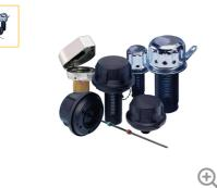
The Parker AB Series comprises a broad range of topmounted breathers and filler breathers. The filler breathers protect hydraulic systems from airborne particle ingress, while allowing sufficient airflow into and out of the fluid reservoir.
