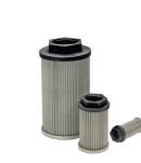
The Parker SE Series comprises a range of suction elements / inbuilt tank filters. The elements are equipped with 125 micron rating abs steel wire mesh media and are capable of flows ranging from of 15 - 500 l/min (4 -132 gpm).
