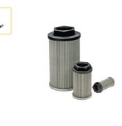
The Parker SE Series comprises a range of suction elements / inbuilt tank filters. The elements are equipped with 125 micron rating abs steel wire mesh media and are capable of flows ranging from of 15 - 500 l/min (4 -132 gpm).
