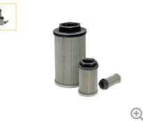
The Parker SE Series comprises a range of suction elements / inbuilt tank filters. The elements are equipped with 125 micron rating abs steel wire mesh media and are capable of flows ranging from of 15 - 500 l/min (4 -132 gpm).
