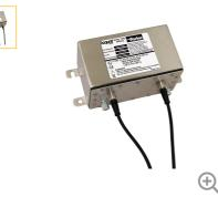
The Parker iCountPD is a highly compact, permanently mounted laser detection particle size monitor that enables continuous monitoring of contamination levels in hydraulic and fluid circuits.Capable of communicating results in ISO4406 / AS4059 or NAS1638.
