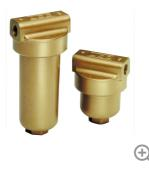
The HPA Series mini high pressure inline hydraulic oil filter is a small, robust filter concept with flow rates up to 45 I/min and pressure level up to 280 bar.
