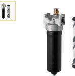
The Parker GMF Series is a highly compact, environmentally friendly inline hydraulic oil filter that features a re-usable element core. Capable of flows up to 600 L/min (158 GPM). Maximum allowable operating pressure 70 bar (1,015 psi).
