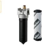
The Parker GMF Series is a highly compact, environmentally friendly inline hydraulic oil filter that features a re-usable element core. Capable of flows up to 600 L/min (158 GPM). Maximum allowable operating pressure 70 bar (1,015 psi).
