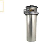
The Parker GLF Series is a tank top return line hydraulic oil filter designed for high flow and long life between element change-outs. Maximum allowable flow 1700 L/min (374 GPM). Maximum allowable operating pressure 10.3 bar (150 psi) static.
