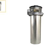
The Parker GLF Series is a tank top return line hydraulic oil filter designed for high flow and long life between element change-outs. Maximum allowable flow 1700 L/min (374 GPM). Maximum allowable operating pressure 10.3 bar (150 psi) static.
