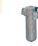
The In-line GA series low pressure filters feature magnetic pre-filtration and a wide range of filter media. A light weight aluminium housing design, with maximum flow rate of 320 l/min and a maximum pressure of 30 bar.
