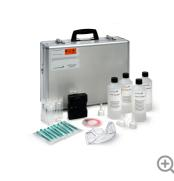
Measure both the weak organic and strong inorganic acids present within an oil with the Parker TAN Drop Test. The result is shown by a colour change, providing you with easy to interpret results, suitable for use by non-technical personnel.
