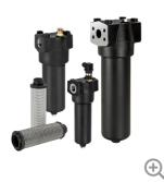
The Parker EPF Series is a highly compact, eco-friendly inline hydraulic oil filter that features a re-usable element core. Capable of flows up to 700 L/min (185 GPM). Maximum allowable operating pressure 450 bar (6,500 psi).
