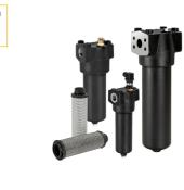
The Parker EPF Series is a highly compact, eco-friendly inline hydraulic oil filter that features a re-usable element core. Capable of flows up to 700 L/min (185 GPM). Maximum allowable operating pressure 450 bar (6,500 psi).
