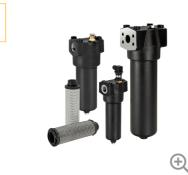
The Parker EPF Series is a highly compact, eco-friendly inline hydraulic oil filter that features a re-usable element core. Capable of flows up to 700 L/min (185 GPM). Maximum allowable operating pressure 450 bar (6,500 psi).
