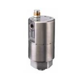
EAPF iProtect® stainless steel in-line filter series is designed to provide high quality filtration of hydraulic systems in marine, oil and gas and process equipment markets covering a flow range up to 120l/min at max 690 bar pressure level.
