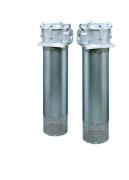
The BGT Series features pre-filtration by means of a magnet column and a full flow bypass with low hysteresis. Providing maximum flow rates of 2400 l/min at maximum pressure 10 bar.
