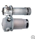
ATZ Series Suction Filters. Submersible (under oil level) tank-wall mounted suction line filters containing a valve that closes automatically before changing the element. Maximum flow 300 l/min.
