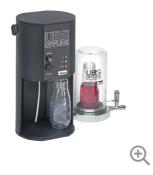
Simple and efficient offline oil sampling, ideal for batch oil sampling.
