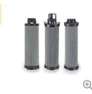
Parker EPF Series Replacement Elements are designed for use with EPF Series High Pressure Inline Hydraulic Oil Filters. Multiple filtration media options available down to 2 microns. Maximum allowable flow 700 L/min (185 GPM).
