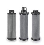
Parker EPF Series Replacement Elements are designed for use with EPF Series High Pressure Inline Hydraulic Oil Filters. Multiple filtration media options available down to 2 microns. Maximum allowable flow 700 L/min (185 GPM).
