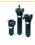
High pressure inline hydraulic oil filter series is a proven filter concept, with multiple connection options up to 500l/min and pressures up to 420 bar.
