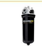
The Parker 12CS/50CS Coreless Medium Pressure Spin-On Filter Series are the Smart Alternative to Spin-on Cans. Max allowable operating pressure of 500 PSI/34.5 Bar and capable of flows up to 50 GPM/190 LPM depending on viscosity.
