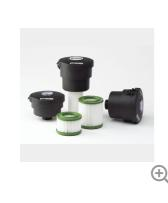
The Parker EAB Series is an eco-friendly reservoir breather / air filter suited for a wide range of hydraulic system applications. Multiple filter media options available down to 1 micron abs. Designed for airflows up to 1500 L/min (396 GPM).
