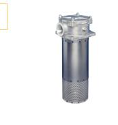
The TTF Series features pre-filtration by means of a magnet column and a quick response bypass with low hysteresis. Maximum pressure 10 bar. Maximum flow 500 l/min. A second return port is an available option as is a filling port in the filter cover.
