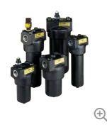
18/28/38P high pressure inline hydraulic oil filter series is a globally proven filter with optimised sizing covering flows up to 700 l/min and a pressure level up to 414 bar.
