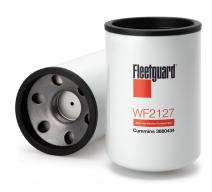
**Thread Size** M36 X 2-6G INT **Additive Base Borate Nitrite Largest OD** 95.76 mm Length 146.30 mm Seam OD 95.76 mm **Chemical Additive** NONE **Gasket OD** 95.76 mm **Gasket Inside Diameter** 80.87 mm
