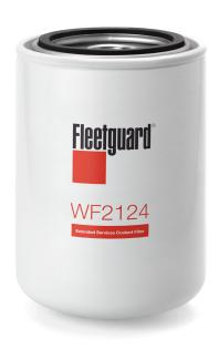
**Thread Size** 3/4-20 UNEF-2B **Additive Base** DCA4+ Largest OD 93.73 mm **TABLET COOLANT ADDITIVE FORM** Length 137.92 mm **Gasket Inside Diameter** 62.53 mm **Gasket OD** 71.98 mm Seam OD 93.78 mm DCA4+ **Chemical Additive**
