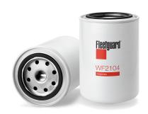
Largest OD93.12 mmCOOLANT ADDITIVE FORMPELLETLength137.59 mmAdditive BaseDCA4+Thread Size11/16-16 UN-2BGasket Inside Diameter62.53 mm
