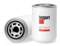
Length 150.00 mm **BPV OPENING DP** No **Thread Form British Largest OD** 96.00 mm **Gasket Inside Diameter** 61.50 mm Gasket OD 71.50 mm **Hydrostatic Burst Minimum** 2000 kPa Thread Type Internal Flow Direction Outside In
