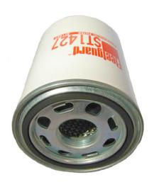
Yes **BPV OPENING DP** Length 181.00 mm Thread Form British **Largest OD** 128.00 mm **Gasket Inside Diameter** 98.00 mm 107.00 mm **Gasket OD Hydrostatic Burst Minimum** 1500 kPa Particle Size at Beta 75 12 micron Internal Thread Type Flow Direction Outside In
