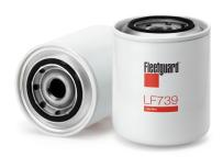
**Gasket Inside Diameter** 62.23 mm **Gasket OD** 71.27 mm **Thread Size** 1-16 UN-2B 131.06 mm Length 107.67 mm Largest OD **BPV OPENING DP** 0 kPa
