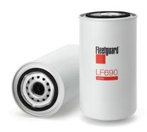
**Gasket Inside Diameter** 62.53 mm **Gasket OD** 71.98 mm 1-12 UNF-2B Thread Size 175.18 mm Length **BPV OPENING DP** 69 kPa Largest OD 96.06 mm Seam OD 96.06 mm **Efficiency** 83% NO Standpipe **Anti Drain Back Valve** Yes **Length / Overall Height** 175.18 mm
