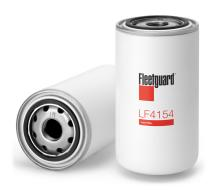
Gasket Inside Diameter 62.00 mm **Gasket OD** 70.00 mm **Thread Size** 1-12 UNF-2B Length 174.10 mm 93.50 mm **Largest OD BPV OPENING DP** 250 kPa Seam OD 93.50 mm **Efficiency** 55% **Standpipe** NO
