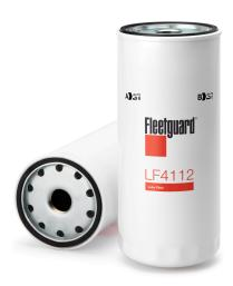
**Gasket Inside Diameter** 92.20 mm **Gasket OD** 100.20 mm **BPV OPENING DP** 250 kPa 108.00 mm **Largest OD Thread Size** 1 1/8-16 UN-2B 260.50 mm Length Seam OD
