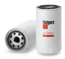
**Gasket OD** 71.98 mm **Gasket Inside Diameter** 62.53 mm Largest OD 94.44 mm **BPV OPENING DP** 139 kPa Length 175.26 mm 1-12 UNF-2B Thread Size 94.23 mm Seam OD **Efficiency** 95% NO Standpipe **Anti Drain Back Valve** No
