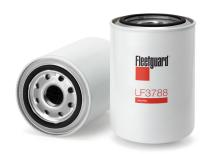
**Thread Size** 1-12 UNF-2B 93.78 mm Largest OD **BPV OPENING DP** 152 kPa 137.60 mm Length **Gasket Inside Diameter** 62.53 mm Gasket OD 71.98 mm Seam OD 93.78 mm **Efficiency** 100% NO **Standpipe Length / Overall Height** 137.60 mm
