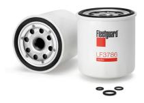
**Gasket OD** 86.00 mm **Gasket Inside Diameter** 75.01 mm **Thread Size** M20 X 1.5 INT **BPV OPENING DP** 103.4 kPa Largest OD 89.99 mm 103.00 mm Length Seam OD 94.01 mm 95% **Efficiency** NO **Standpipe**
