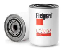
Gasket OD70.00 mmGasket Inside Diameter62.00 mmLength144.20 mmLargest OD108.00 mmBPV OPENING DP250 kPa
