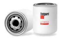
**Gasket Inside Diameter** 62.00 mm **Gasket OD** 70.00 mm **BPV OPENING DP** 160 kPa Length 116.10 mm 93.50 mm Largest OD Thread Size 1-12 UNF-2B Seam OD 93.50 mm **Efficiency** 55%
