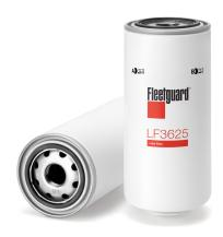
Largest OD 93.50 mm **Thread Size** 1-12 UNF-2B 216.30 mm Length **BPV OPENING DP** 250 kPa **Gasket Inside Diameter** 62.00 mm **Gasket OD** 70.00 mm Seam OD 93.50 mm **Efficiency** 55% **Standpipe** NO
