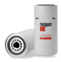
Gasket OD 71.98 mm **Gasket Inside Diameter** 62.54 mm **Thread Size** 1-12 UNF-2B Length 204.72 mm 96.09 mm **Largest OD BPV OPENING DP** 0 kPa Seam OD 96.01 mm 100% **Efficiency** YES Standpipe Length / Overall Height 204.60 mm
