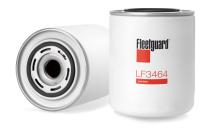
Thread Size 1-12 UNF-2B **Media Type** StrataPore 135.50 mm Length **Largest OD** 108.00 mm **BPV OPENING DP** 160 kPa **Gasket Inside Diameter** 62.00 mm **Gasket OD** 70.00 mm Seam OD 107.50 mm **Efficiency** 75% NO
